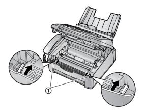
7 Close the front cover (①) by pushing down on both sides, until locked.
